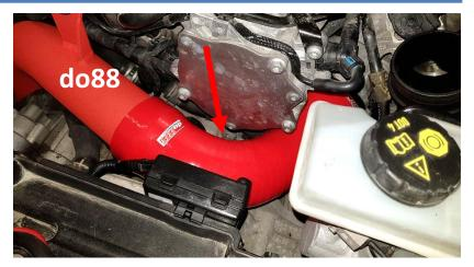
Remove 3x Allen screw 5mm.
