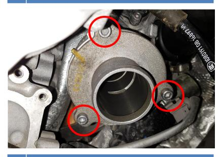
6. Install the do88 turbo muffler delete with the screws removed in step 4.
