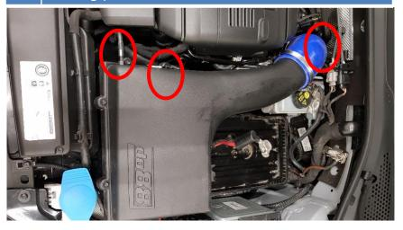
3. If you have OEM intercooler pipes: Loosen 1x Torx T30 screw at the pressure pipe bracket and remove the hose at the turbo outlet. Also disconnect the small plastic box from it bracket on the battery tray. Gently pull away he pipe now to make space at the turbo outlet.
