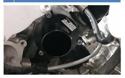
**5.** Check that the O-ring still sits correctly in the turbo housing.
