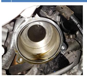
7. Install the included silicone hose and hose clamps inbetween the turbo muffler delete and the intercooler pipe. Install all other parts in reverse order.
