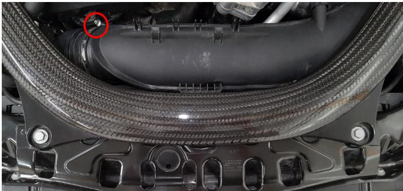
8. Remove this plastic/rubber bracket which is holding the inlet pipe, by twisting the rubber 90 degrees and lifting it up. Now you can remove the whole intake pipe and filter box.
