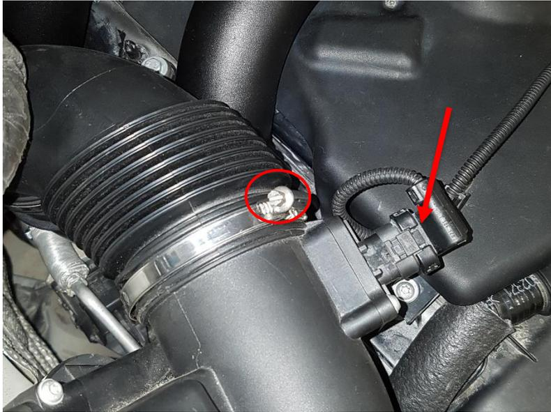
10. Install the two AMM sensors to both do88 pipes with included M4x12mm Allen screws.
