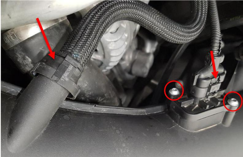
6. Remove the coolant hose from the inlet pipe.
