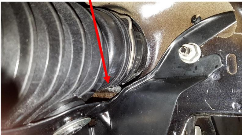
**14.** If you have bought the do88 Performance Y-pipe to fit together with the do88 Performance intercooler setup. Now install both intercooler outlet silicone hoses. It is easier if you put the hose clamp on the intercooler outlet before pushing on the silicone hose.
