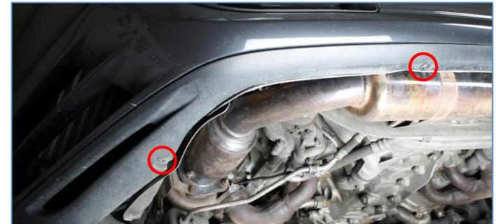
7. Remove the Torx T30 in each wheel arch the holds the upper edge of the bumper from underneath.
