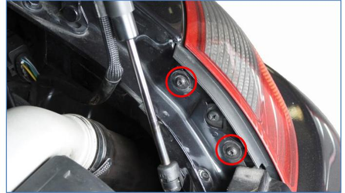
2. Remove 1pc Torx T30 plastic lock screws from the plastic clips on each side of the car located in the front of the space for the rear lights. Then pull out plastic clip.
