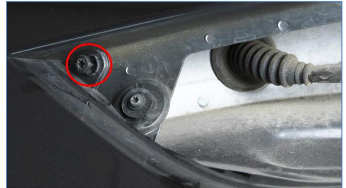
3. Remove 4pc Torx T30 screws located on the top of the rear bumper.
