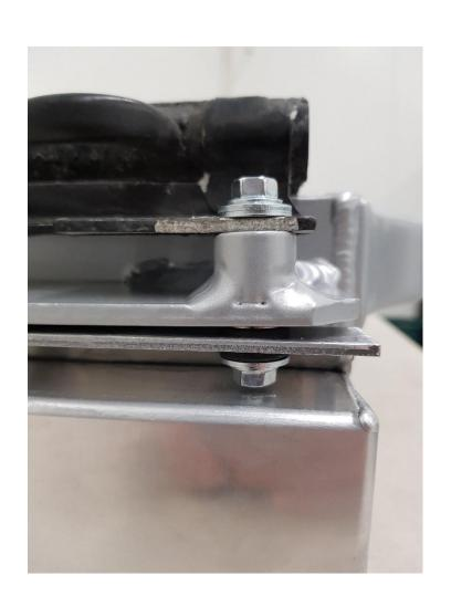
When the do88 aluminum radiator is installed together with the intercooler you must install it with the included hardware kit.
