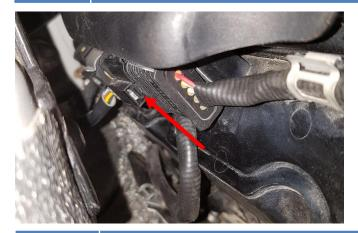
Disconnect the connector from the O2 sensor located on the rear downpipe with the help of a small flathead screwdriver and carefully separate the plastic tabs.
