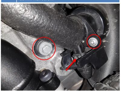
Remove 1x 10mm hex screw from the rear pipe. Separate the plastic pipe from the turbo connector to get more space. Remove the rubber grommet and install it on the do88 pipe.
