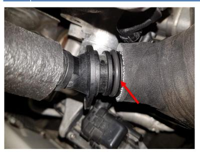
Assemble the do88 pipe with the orange OEM O-ring and also the included O-ring.
