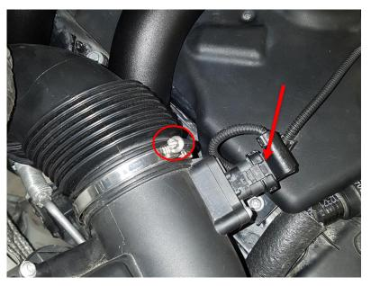
10. Remove 1x Torx T25 screw on plastic bracket, located on the front pipe.
