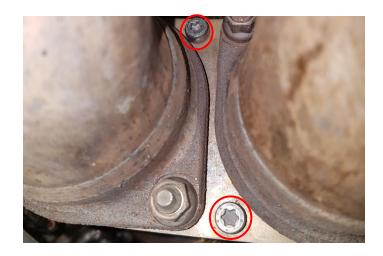
Remove the O2 sensor from front downpipe with a 22mm 02 socket. and the V-band with a 13mm hex, use a larger flathead screwdriver to separate the V-band.
