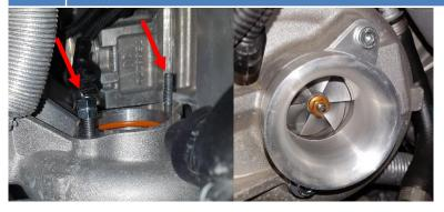
Remove the 2x hex 10mm and 2xTorx T30 that's holding the inlet pipes on the turbo chargers.
