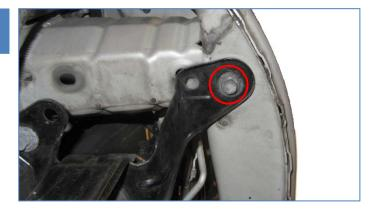
14.Install left and right intercooler bracket with 1pc M8x30 flange<br/>head screw and a thick washer each. The thick washer installs<br/>between the bracket and the radiator bracket.<br/>Do not tighten screws now as brackets should be adjustable.
