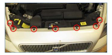
**4.** Pull the rear end of bumper out from the car until it comes loose on both sides of vehicle.
