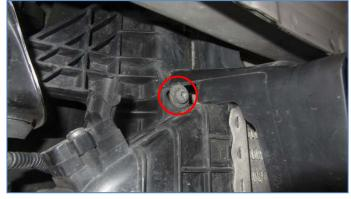
**12.** Remove the sensor from the OEM intercooler by removing its Torx T25 screw and pull it up from the intercooler.
