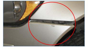
**5.** Pry the plastic fastener that attach the front protecting plate to the radiator frame and pull the bumper a bit forward so it will not attach again.
