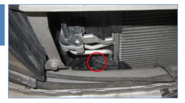
**10.** Remove both hose ends from the intercooler by loosen the hose clamps with an 7mm hose clamp screwdriver or 7mm hex socket and then pull the hose ends of the intercooler connections. The hoses can remain installed on car during this job if you should not replace them at the same time.
