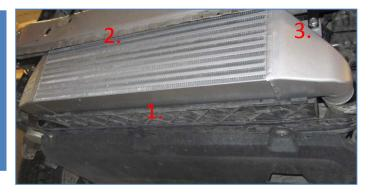
16. Adjust the position of the intercooler while brackets are loose until the grooves aligns with the screw boss for OEM intercooler and have contact with them. The lower edge of the intercooler should be about 3mm (1/8") from the radiator plastic frame according to picture. Hold the intercooler in this position and tighten the two screws to the vehicles bumper beam and the screws and nuts between intercooler and bracket.
