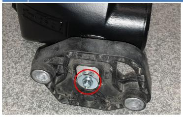
Remove both intercooler mounts from intercooler by prying locking tabs seen from bottom of intercooler using a screwdriver then remove locking plates and slide mounts off the intercooler.
