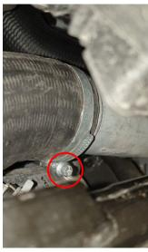
Install the intercooler mounts on the do88 intercooler, in same direction as it had on OEM intercooler. Secure in place using 1pc 5,5x22mm washer and 1pc M5x12mm Allen screw on each side.
