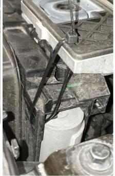
13. Loosen the fan cover by pressing in the locking tabs on both sides, then lift the fan cover about 2cm (3/4") upwards. Leave it in this position.
