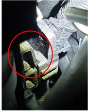
**15.** Remove 2pcs 10mm hex screws on each side that holds the intercooler mounts.
