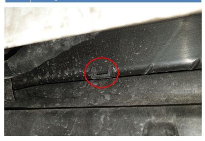
**18.** Disconnect shutter motor connector and the cable holder that sits in the air guide.
