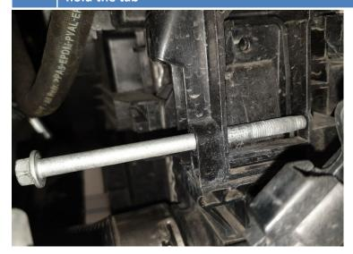
Pry here with a screwdriver to separate the intercooler. Then remove intercooler from car by first lowering the right side until the left side slides out of its bracket. Be aware of the lower left fan cover bracket so you don't damage it.
