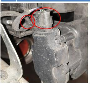
20. Disconnect cable connector from right side horn and then loosen the 8mm hex screw and remove horn from car.
