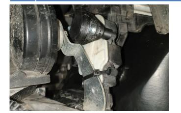
Assemble the actuator to the grille shutter limiter with the T-shaped rotation limiter as close as possible to the rotation just determined. Secure with 2pcs 5x25 screws included, screw in slowly to avoid damages to the actuator housing.
