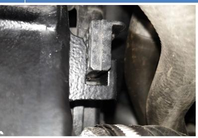
On S90/V90 and some other models it might be necessary to cut the corners of the upper air guide according to before and after pictures below.
