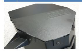
9. Install the do88 air box in vehicle by lowering it in place in the rubber grommets, mount the hose on the air mass meter housing and tighten its hose clamp.
