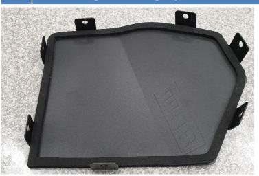
8. Optional! If you prefer more intake sound it is possible to use the air filter system without the lid, but this will also increase the intake air temperature a bit.
