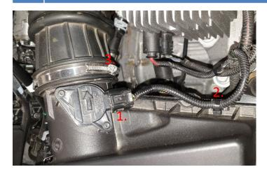
Remove the air mass meter sensor from housing by removing 2pcs Torx T20 and lift it up.
