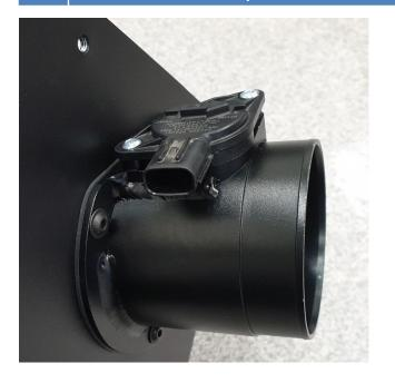
Install the included Edge sealing strip on the air filter housing according to picture.
