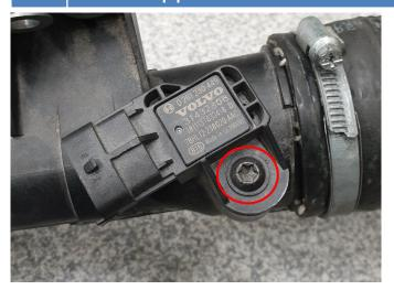
Install sensor in do88 intercooler pipe and secure **17.** with supplied M5x12 Flange screw
