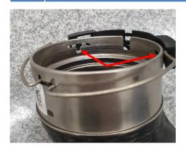
Install the sealing ring and lock clips in the included Henn 20. connector adapters. Make sure the sealing ring is installed in the same direction as it was in the OEM hose.
