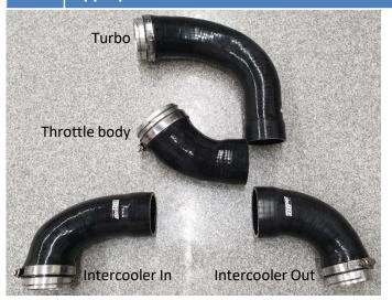
22. Install hoses on intercooler, Turbo and throttle body.
