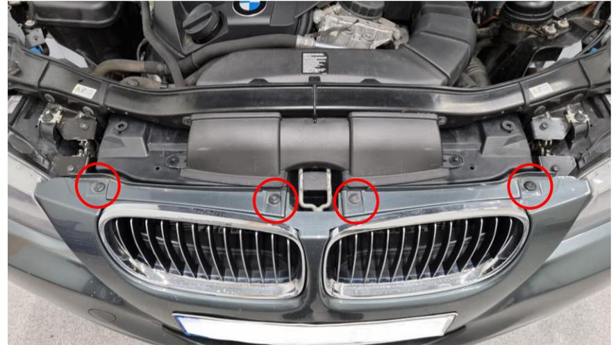
8. Now remove the front bumper and then remove 9x Hex 8mm screws from the "under engine cover" and then remove this cover.
