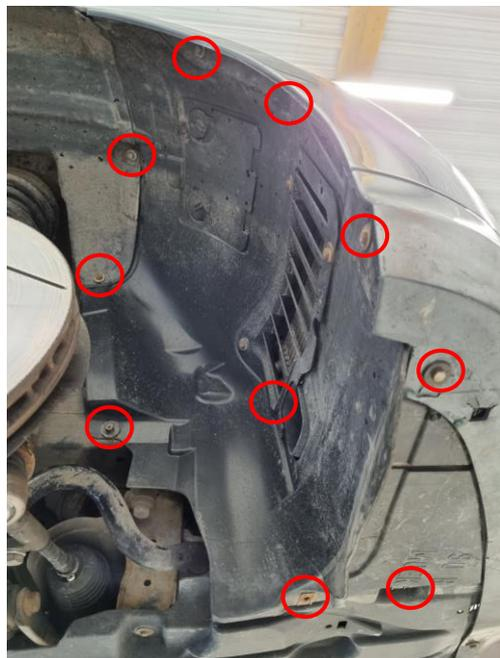
5. Remove 2x Hex 8mm Screws in each upper corner of the bumper on both sides.
