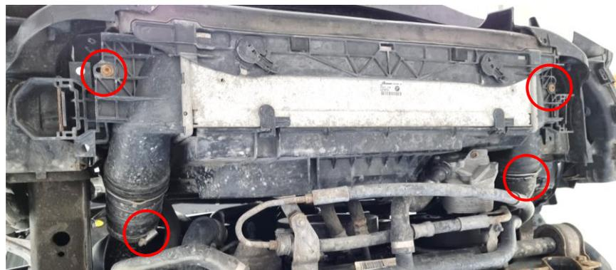
**10.** Remove the intercooler outlet charge pipe. Loosen 1x hose clamp.
