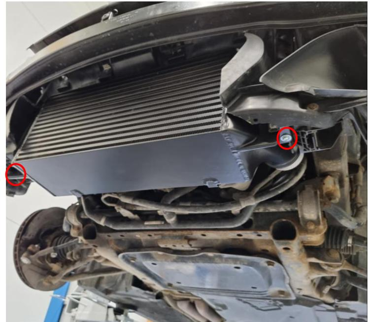
14. Attach the included plastic air guide. Fasten it as on the photo\* below with the included sheet metal screws. You can access the screws if you pry out the air guide behind the kidney grill.
