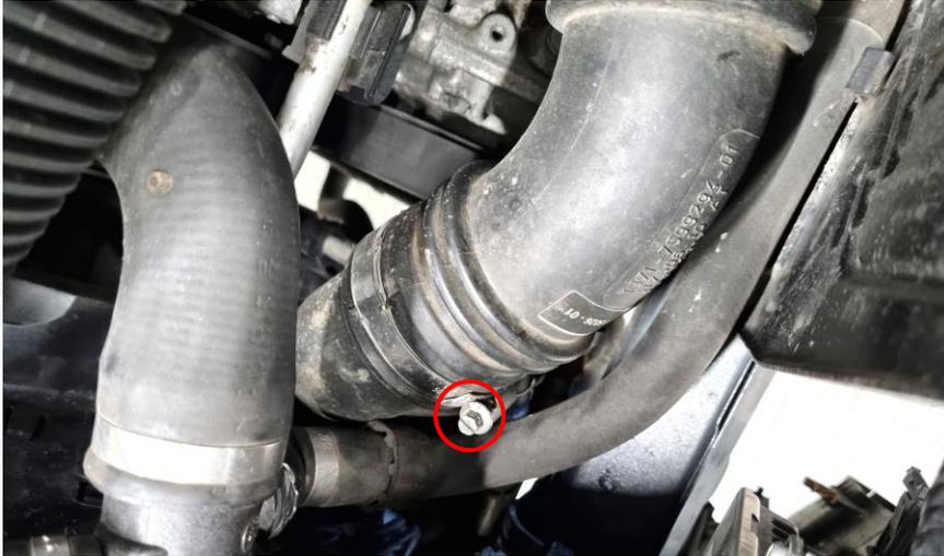
**11.** Trim the plastic according to the marked areas on the photos below. Not you will need to relocate the ambient temperature sensor marked on the right-side photo (Fasten it with the included zip-tie).
