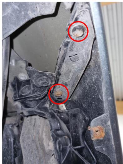
6. Remove 3x Hex 8mm screw along the bottom of the front bumper.
