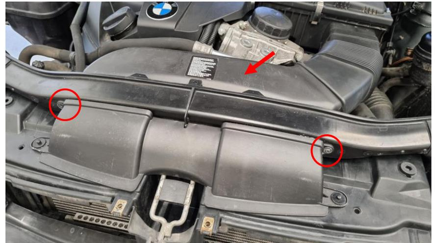
16. Remove the charge pipe screw 1x Torx T30.
