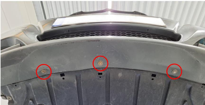
7. Remove 4x Torx T30 screws along the top of the bumper.
