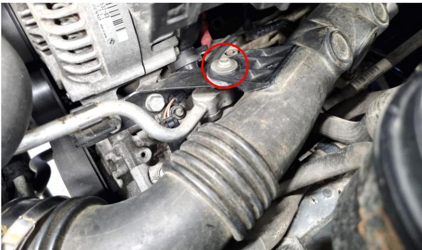
17. Attach the included intercooler outlet silicone hose on the intercooler. Then install the included aluminum charge pipe from the top (red on this photo).
