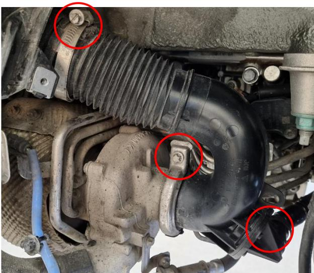
**24.** Loosen the turbo outlet hose clamp.
