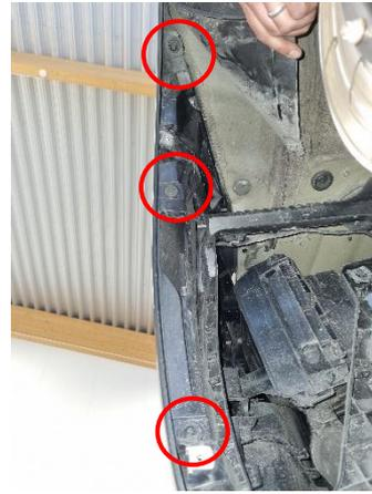
**15.** Remove 2x Torx T30 located top center of the rear bumper cover.
