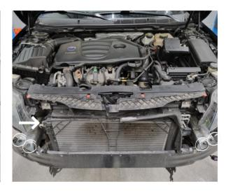
Remove Torx E12 screws on both sides of the car. Disconnect washer fluid hose and plug the reservoir with the included 12mm silicone cap. Unplug the cable to fog lights and sensors. Remove front bumper with the help of an assistant.
