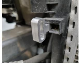
Remove clamps with a 6mm hex screwdriver and disconnect the intercooler pipes on both sides. Use a flathead screwdriver and gently push the plastic tabs to separate the intercooler from the radiator. Lift it out of the car.
