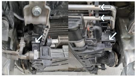
Remove screws x4 to remove plastic air guide.
