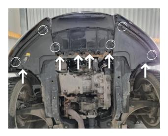
Step 3 Remove screws x6 and use a flathead screwdriver to remove plastic tabs x2.
